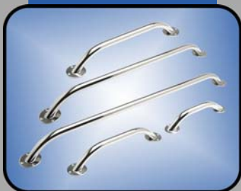
SS Flange Mount Handles Polished stainless steel grab handle with a 3 screw mounting flange. Flange O.D. is 2 3/8". GH-FM8 8" GH-FM12 12" GH-FM16 16" GH-FM24 24" GH-FM36 36"
