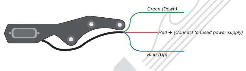
Wiring instructions for use with the Dana Marine Steering Trim Switch w/Coil Cord Optional Wire Loom
