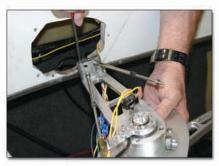
18. Re-attach anchoring point to the shifter arm. If using a 33c cable use supplied cable ends to attach cables to pivot arms. Mercury style cables do not require cable ends to make this attachment.
