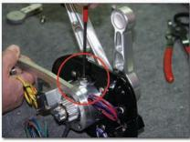
21. The neutral detent adjustment is set from the factory to the correct specs. You can adjust it to your feel, but over tightening can cause detent failure.
