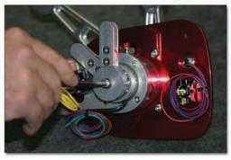
Remove center bolt to remove the shifter pivot arm.
