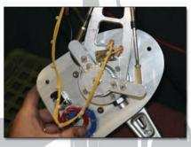
20. Before final installation be sure to check cable arm movements to ensure proper cable actions for throttle and shift.
