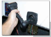
1. Remove stock shifter, this process will vary depending on the control you are removing.
