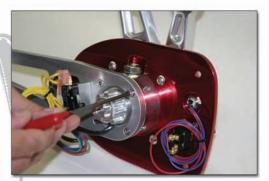
Remove the 4 larger allen bolts to remove the shifter arm.
