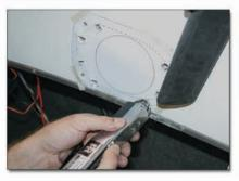
Now with all of your holes drilled, using an air saw or a jig saw, cut on the dotted line to create the proper opening for your shifter.
