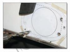
8. With the cutting template taped into place, start by drilling the mounting holes by using a 1/4" drill bit. Next drill your cutting pilot holes using a 1/2" drill bit.
