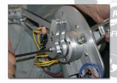
13. When attaching pivot arms take special care in making sure that the arms will provide proper movement, as required for your throttle and shift.
