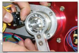
Be very careful when removing and installing the shifter pivot arm not to damage the neutral safety switch.
