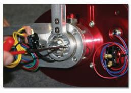
Remove the 4 allen bolts to remove the throttle pivot arm.
