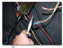
Before clipping the stock wiring be sure to mark each wire with the correct function to avoid confusion when re-wiring.
