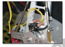
19. Notice that all of the wiring is tie wrapped out of the way to avoid any moving parts, this is a must.
