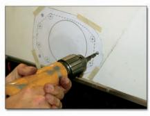
7. BEWARE. Before cutting or drilling any holes, be sure there is a minimum of 3 3/8" of clearance behind the shifter mount plate.
