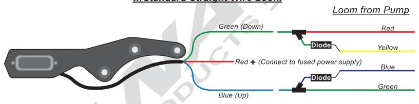
Wiring instructions for use with the Dana Marine Steering Trim Switch w/Coil Cord Optional Wire Loom
