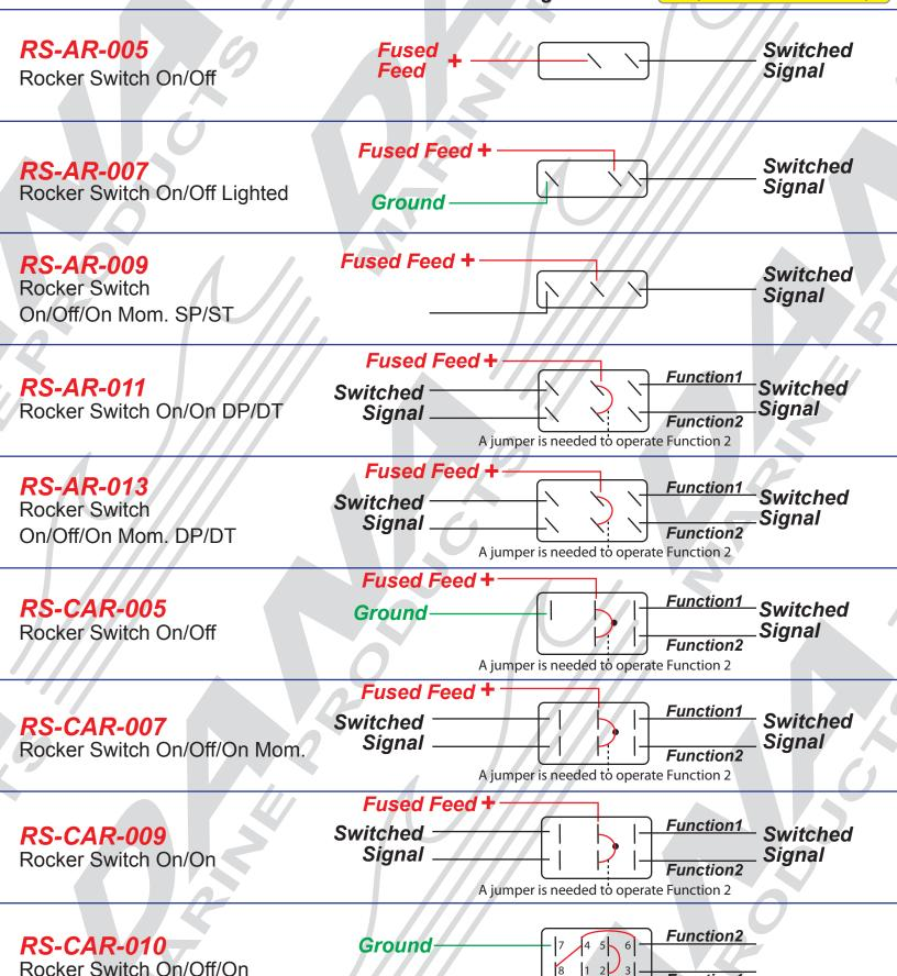
Typical installation for: Nav. Lights/Dash Lights or Bilge/Auto Bilge. Activating the switch in one direction operates a single function, activating the switch in the opposite direction operates both functions.
