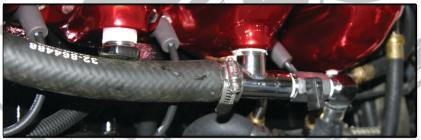
With sealant applied, install drainback valve with the valve handle facing outward. Next install the 90 deg. fitting, it is necessary to turn the lower SS fitting outward to thread in the 90 deg. fitting. Once tight, return the assembly back to a straight position.
