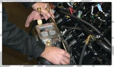
With the manifold loosely in place Install the remaining manifold route the oil lines behind. Be sure bolts and tighten to 25 ft. lbs. that the rubber line is below the stainless line. Be sure not to pinch the drive reservoir line between the valve cover and manifold.
