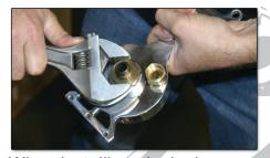
When installing nipple, be sure seals are seated properly and not being crushed. Also install provided oil line adapter fitting using Teflon sealer.
