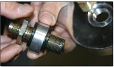
Using the provided spacer, o-ring, and stock oil seal re-install nipple into new DMP head. Install oil seal on top & bottom of the spacer
